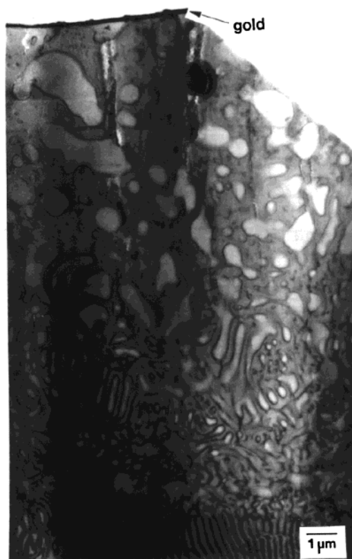
Figure 12. Cross-sectional TEM micrograph (OsO 4 stained) of the near-surface morphology of an SB 80/80 diblock copolymer sample showing the complex morphology with a contaminant thought to be a fully polymerized PS block with varying lengths of PB. The external surface has been marked with a layer of gold. The normal lamellar structure is ~10 μm below the surface. Reprinted with permission from ref 31. Copyright 1992 Massachusetts Institute of Technology. Courtesy of E. L. Thomas, Massachusetts Institute of Technology, Cambridge, MA.
